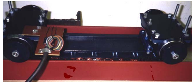
Fig. 9. Single sided PM LSM with moving 3-phase primary.
