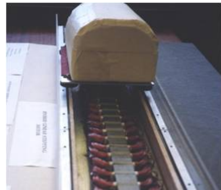
Fig. 25. Prototype of a LIM-driven people mover with permanent magnet repulsive suspension system.
