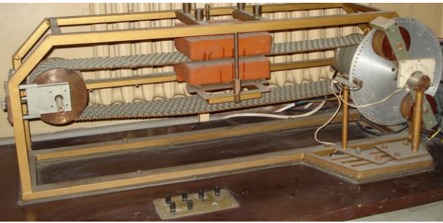
Fig. 7. Laboratory equipment with double-sided LIM with elastic secondary for testing a small-scale LIM-driven belt conveyor.
