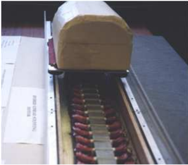
Figure 17. Prototype of a LIM-driven people mover with permanent magnet repulsive suspension system.
