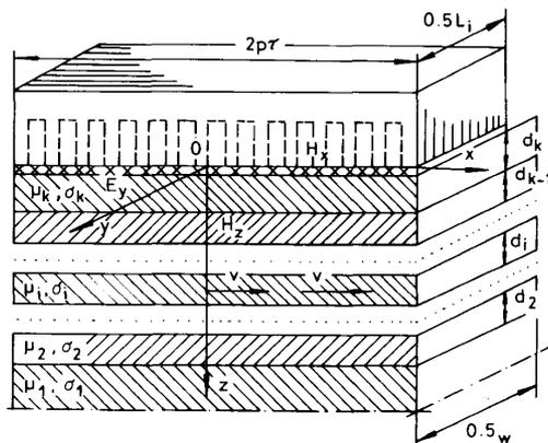
Fig. 1 Model of a multilayer rotor induction machine in Cartesian co-ordinate system for analysis of electromagnetic field
