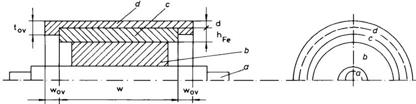
Fig. 5 Double-layer low-inertia rotor with distributed parameters
