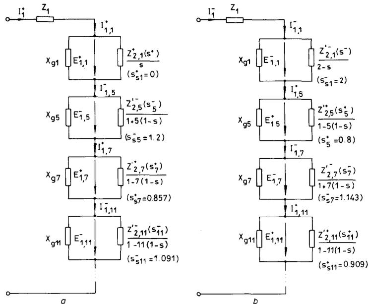
Fig. 3 Equivalent circuits for multilayer rotor induction motor under unbalanced conditions
