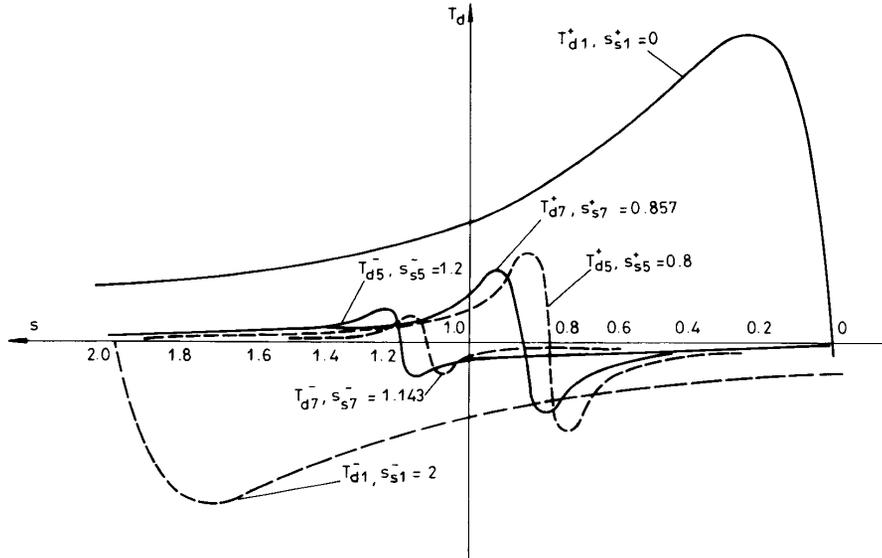
Fig. 4 Torque-slip curves for higher time harmonics  $v = 1, 5$  and  $7$
