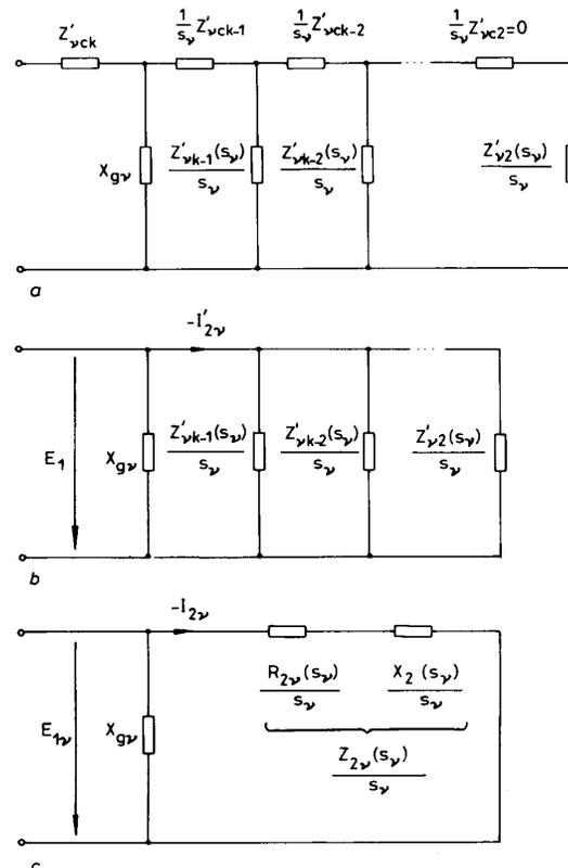
Fig. 2 Circuit models for multilayer rotor with distributed parameters
