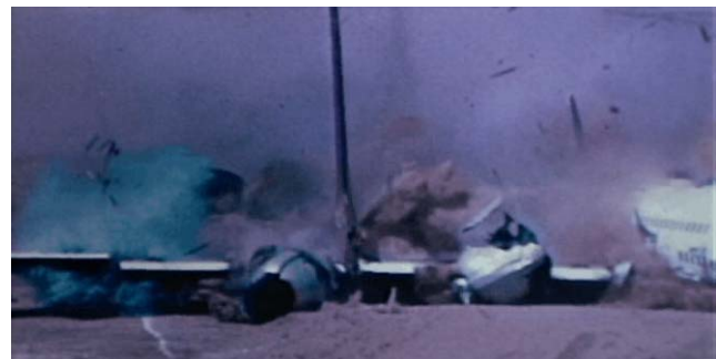
Fig. 3. LC-1649 full-scale dynamic crash test. Inboard pole impact [6].
