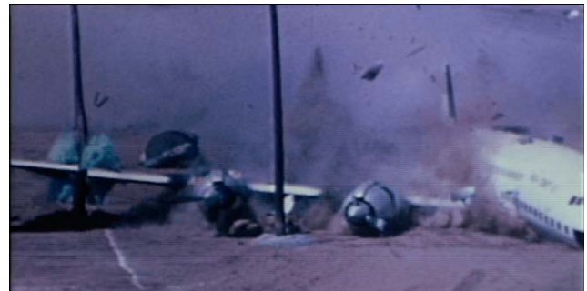
Fig. 2. LC-1649 full-scale dynamic crash test. Outboard pole impact [6].
