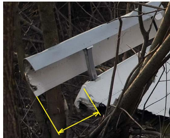
Fig. 11. Tip of the left wing. The wing has been cut off while the slat is intact. http://vfl.ru/fotos/aa582e8c473661.html
